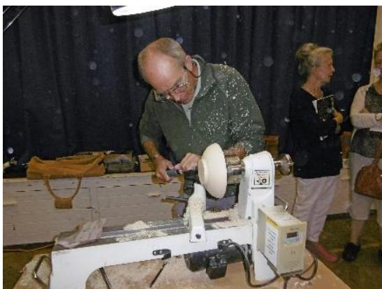
Mike mounted a piece of Sycamore on a screw chuck and started to shape the outside of a small bowl. He then reversed it into a four-jaw chuck and hollowed out the inside. He showed how you can, with good tool technique, get a good finish straight from the tool. The advantage of this is that it requires less sanding to get the final finish.
